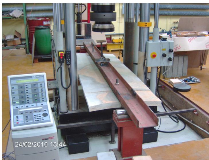
*Figure 6: Testing of the 2.1 x 0.8 x 0.05 m panel cut out from the reference wall. Spacing of anchors 0.8 m, the load distributed by the C-channel in the centre (photo auth.)*
