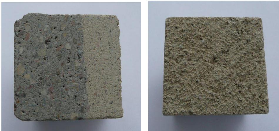
*Figure 4: Shotcrete samples: double-coating concrete with an external pale yellow architectural coat made according to „cut” technique (photo auth.)*
